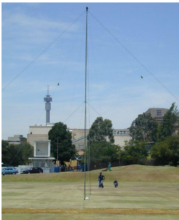
Antenna mounted on 10 m mast
